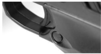
Press the safety button until the red mark disappears. Now the trigger is blocked.
